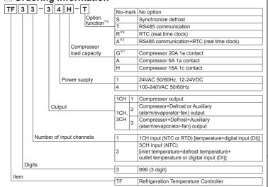
$\times$ 1: Only for 1CH input, compressor output model (TF31-1 $\square$ G).
