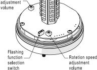
F1: 80±10times per minute F3: 240+10times per minute ( emergency signal display light )
