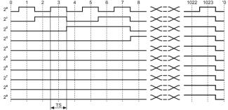
XTS=0.3515625°±15' \*Above waveform is based on the positive logic. (The output waveform of negative logic is in reverse.)
