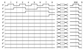
XAbove waveform is based on the positive logic. (The output waveform of negative logic is in reverse.)
