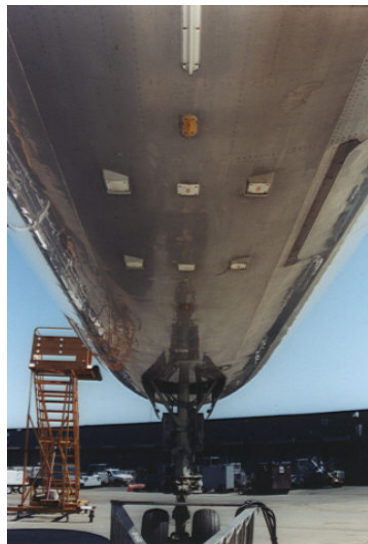
Fig. 6-7 Triple LRRR Antenna Installation (ARINC square patch type)
