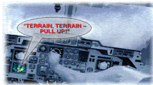
Fig. 6-16 Terrain Awareness and Warning System
