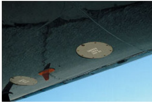
Fig. 6-8 LRRRA Antenna Installation (recessed horn type)
