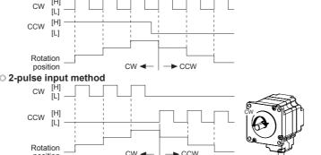
\*Do not input CW, CCW signals at the same time in 2-pulse input method. It may not operate properly if another direction signal is inputted when one of CW or CCW is [H].
